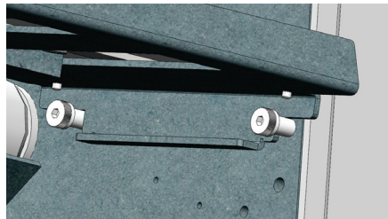
Figure 5: Lower Fold Plate in Proper Position
