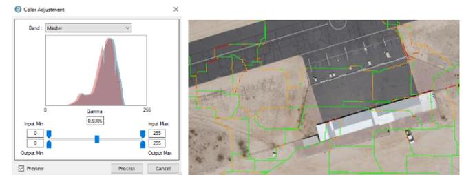
Automatically generated mosaics can be interactively edited using the mosaic editing module. This allows for manual modification of seamlines with real-time visual feedback on the effect of changes.
