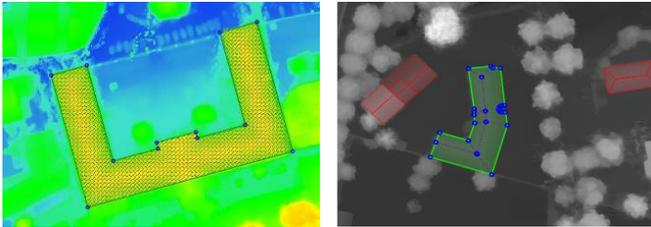
The feature extraction module enables the user to extract 3D features from a DSM by creating 3D polygons. Automatic contour detection of buildings and other features enable fast footprint collection. This semi-automatic design saves time over traditional vector extraction methods.
