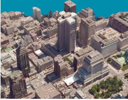
Correlator3D™ can generate photorealistic 3D models. The process creates a mesh from a DSM, then uses input images to texturize it. The size of the output model is determined by the user.
