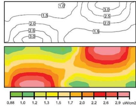
Figure 6: Contour and heat map from light simulation of UVM 222 EXC onto conference table
