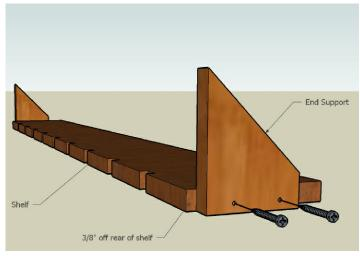
STEP 5. ATTACH END SUPPORTS TO SHELF. SUPPORT TO BE  $\frac{3}{8}$ " OFFSET FROM REAR OF SHELF. BOTTOM OF SUPPORT TO BE FLUSH WITH BOTTOM OF SHELF
