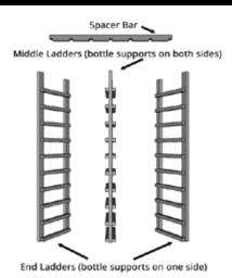
Instructions show a sample 6 column rack. All 38 1/4" Upper Racks are assembled in the same manner. Your order will contain the specific number of ladders and spacer bars appropriate for your chosen rack. Racks wider than 10 columns will have segmented spacer bars with clips to attach them together.
