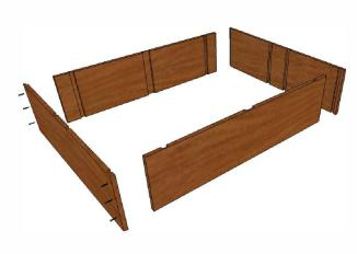
STEP 1. ATTACH TOP AND BOTTOM TO BOTH SIDES WITH (6) SCREWS AS SHOWN
