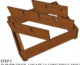
FLIP BIN OVER. LOCATE (1) LONG SHELF AND (2) SHORT SHELVES. SLIDE SHELVES INTO SLOTS AS SHOWN WITH SHELF NOTCHES FACING UPWARD.
