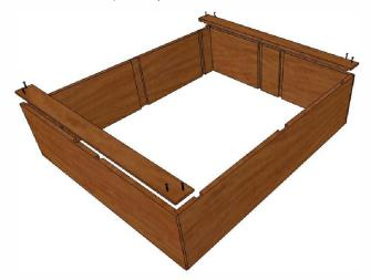
STEP 2. ATTACH LEFT AND RIGHT CLEATS TO BACK OF BIN WITH GLUE AND SCREWS AS SHOWN
