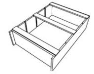
4. Install the back cleats using screws provided. Top & bottom cleats fit flush against top & bottom of shell. Flip over when done.
