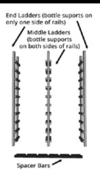
Instructions show a sample 6 column rack. All 39 3/4" Base Racks are assembled in the same manner. Your order will contain the specific number of ladders and spacer bars appropriate for your chosen rack. Racks wider than 10 columns will have segmented spacer bars with clips to attach them together.
