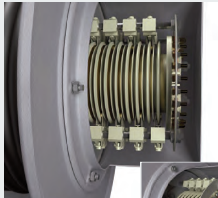
Compact slip ring assembly design with pancake/flat slip ring assemblies 16 A, with collectors & clamp plate
