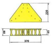
Cable guide set from sheet steel with rollers from shock resistant plastic allowing cable payout in two directions without excessive bending in the cable.
