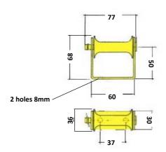
Cable guide from shock resistant plastic with galvanised steel bracket. Useful for reducing cable friction on supporting surface.
