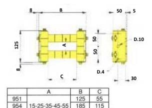
Cable guide from galvanised sheet steel with nylon rollers. Rollers are adjustable to cater for different cable diameters.
