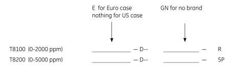
Note: Telaire T8100-R uses the Telaire 6613  $CO_2$  sensor with patented ABC Logic<sup>TM</sup> self-calibration. T8200-R uses the Telaire 6615  $CO_2$  sensor with dual channel self calibration. The calibration interval will depend on the installation environment.
