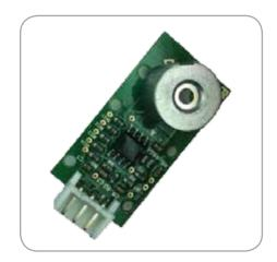
This IR module is used for non-contact surface temperature measuring. The ZTP-315MIH presents the temperature compensated single outputs via voltage output with optics (glass lens for high temperature detection). It can also provide compatibility with the customer's device without the need for recalibration. The ZTP-315MIH uses 3-wire connections: one for output signal, single power supply and ground.
