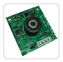
The ZTP-115ML infrared module is used for non-contact surface temperature monitoring. This thermopile IR module presents the temperature compensated single outputs via  $l^2C$  with optics (Silicon Lens). It can also provide compatibility with the customer's device without the need for recalibration. The ZTP-115ML uses 4-wire connections: two signals for  $l^2C$  output, single power supply and ground.
