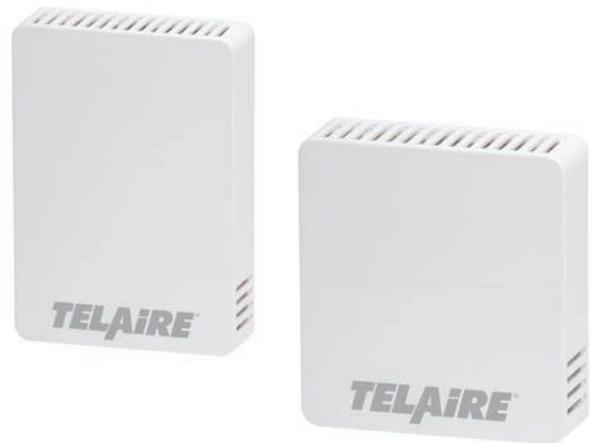
Telaire T5100 Series is a low-cost, high performing CO<sub>2</sub> transmitter for the building controls market. It works seamlessly with building automation systems, and allows you to simply and effectively control fresh air. Demand-controlled ventilation using CO<sub>2</sub> sensors prevents energy losses from over-ventilation while maintaining indoor air quality.
