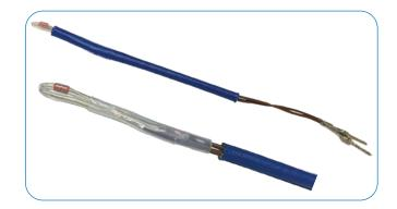
Thermometrics A-1737 Motor Coil Temperature Sensor provides critical temperature feedback of an electric motor's operating condition. Used by either interlacing into the stator coil, or tied to the neutral bus bar on the motor circuit, it provides temperature feedback to indicate motor load or stall conditions.
