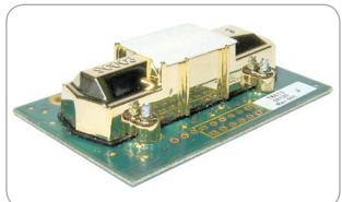
The Telaire T6613 is a small, compact CO<sub>2</sub> Sensor Module designed to meet the volume, cost, and delivery expectations of Original Equipment Manufacturers (OEMs). The module is ideal for customers who are familiar with the design, integration, and handling of electronic components.
