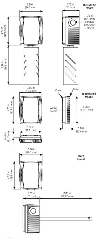
Outside Air Mount Case: ABS flame retardant IP42 rated Space (Wall) Mount Case: ABS flame retardant Duct Mount Case: ABS flame retardant IP42 rated Probe: Stainless steel
