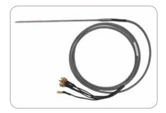
The Type S/AS/ES Thermometrics temperature standards consist of ultra-stable thermistor probes assembled into thin wall stainless steel housings with shielded extension leads. The thermistors used receive special processing to ensure long term stability. All thermistor temperature standards are ruggedly constructed and are suitable for liquid immersion.
