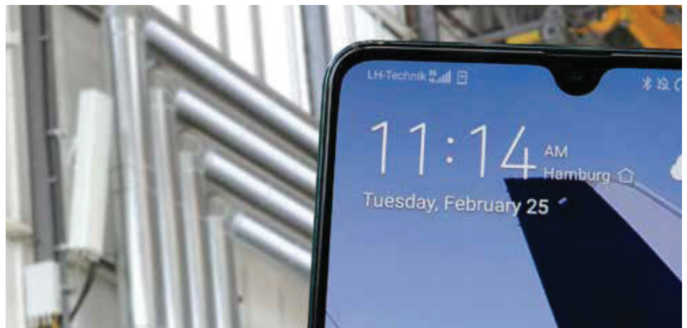
Private – 5G appear as ‘LH-Technik’ on devices; with 5G cell in background (Image: Lufthansa Technik AG/ Jan Brandes)
