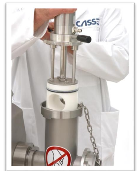
Piston valve for reliable rejection of contaminated product parts.
