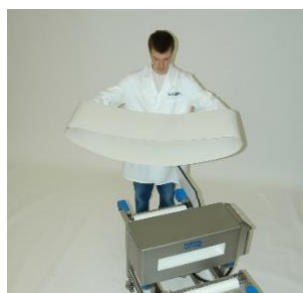
Remove the PU belt completely from the sliding plate.
