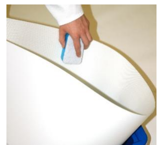
Clean PU belt with a sponge or hose using soap and water.
