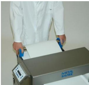
Fold the guide of the deflection roller upwards.
