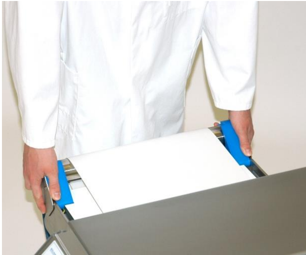
Conveyor HW - particularly easy to dismantle for quick cleaning.
