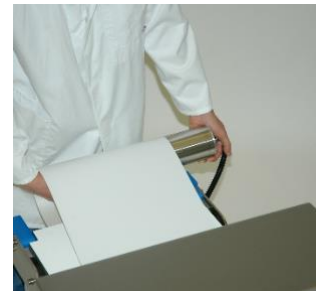
Go to the other side of the conveyor and remove the deflection roller there.
