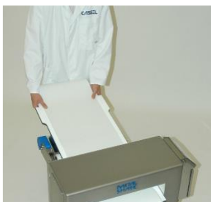
Pull the PU belt as well as the sliding plate out of the unit.
