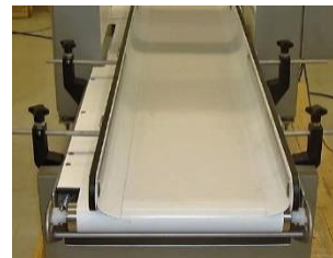
Side rails with silicone lip
