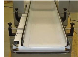
Side rails with silicone lip
