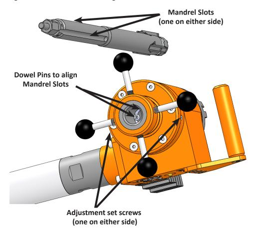
2. Gently feed the mandrel into the cutter head end of the tool (front end) until the mandrel is seated. Once seated, twist the mandrel in a clockwise direction (this will engage the mandrel into the feed wheel's nut). Once the mandrel begins threading into the nut, you may also turn the feed wheel to install the mandrel.
