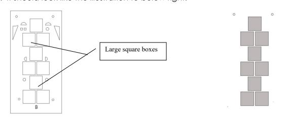
3. Align STENCIL A to painted pavement using alignment holes. Paint whole stencil with colors of your choice. Repeat 1-2 more times to achieve desired vividness, drying after each application, and remove STENCIL A. Let dry. It should like below right.
