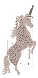
5. The painted stencil on the pavement should appear as below. Take individual letter stencils and align within diamond pattern as desired. Paint and repeat 1-2 more times to achieve desired vividness, drying after each application, and remove each.
