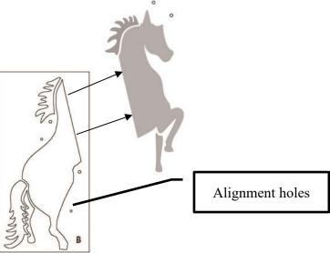
3. Painted stencil should appear on pavement as below left. Align small stencil showing eyes, nose and horn with chalked circular alignment holes as shown to right and paint.
