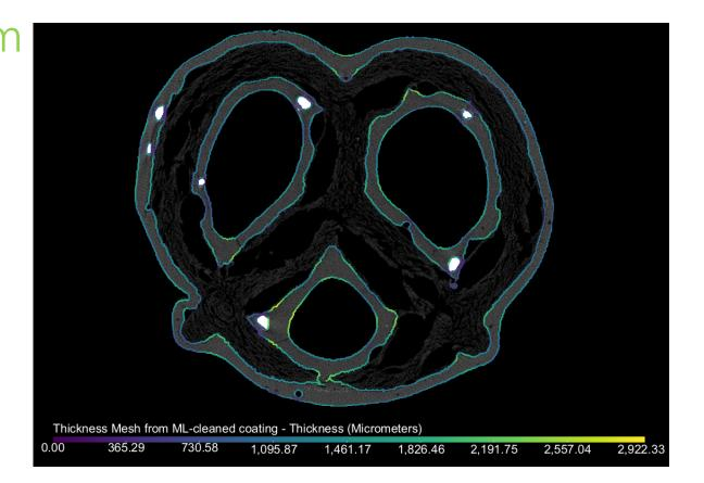
Thickness max 2.9 mm, mean 1.3 mm
