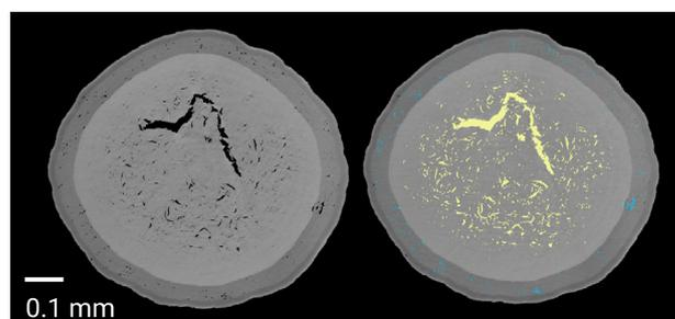
Figure 3: Porosity analysis—in the internal structure of the analyzed particle, a high number of pores were detected, which is reflected by the total porosity of 7.43 percent. Color coding was used according to distance from particle center: Pores in the core layer are yellow and pores in the outer layers are blue.
