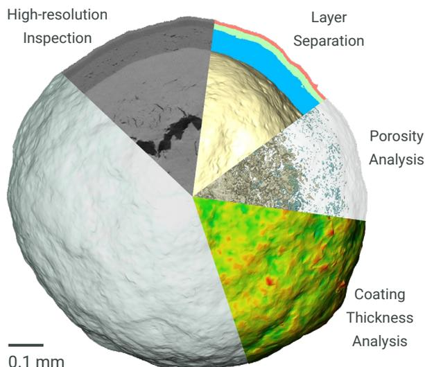
Figure 1: nano3DX particle analysis possibilities.
