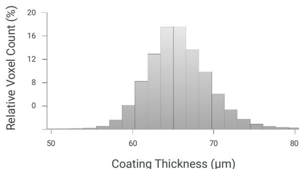
Figure 4: Coating thickness homogeneity analysis—the thickness of the outer coating layer (cellulose acetate layer) of the analyzed particle varied from 50 to 80  $\mu\text{m}$ , reflecting low manufacturing quality.
