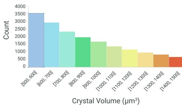
Figure 5: Crystallinity analysis—in the internal structure of the analyzed powder, the crystalline phases were resolvable due to high contrast and resolution. The volume of those phase varied from 500 to 1500  $\mu\text{m}^3$ .
