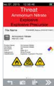
Figures 3 and 4. Analysis of ammonium nitrate through plastic container using Progeny ResQ.
