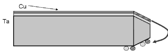
FIGURE 9. Metals adhering to the wafer backside.
