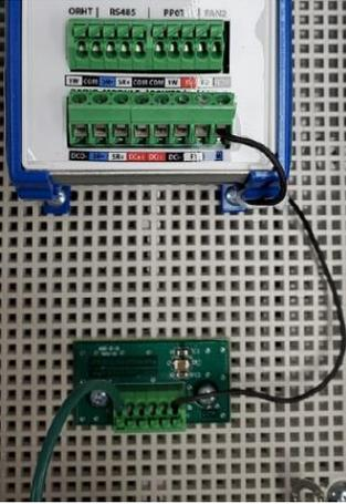
**Note:** All cable runs should be secured in place. It is recommended that the cables from the Fan Node Enclosure to the Fan Control Box be in conduit whenever possible. Additional cables from the Fan Node Radio, Weather Station (ORHT), Plenum Pressure Sensor (PPOT) to the Fan Node Enclosure should have P-Clips to secure them in place if conduit is not used.
