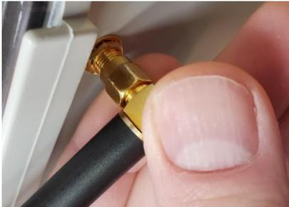
7. Use the supplied (inside the enclosure) 5/16" wrench to secure the antenna in place. Ensure the antenna is always secured vertical to the sky.
