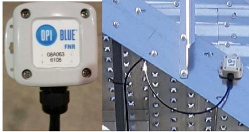
2. Bring the Communication cable (COM2) cable into the Fan Node enclosure through a strain relief and terminate in the proper connection.
