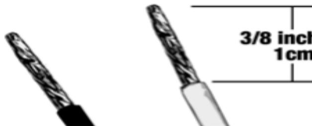
8. Take your strain relief and apply the applicable channel tab and insert the black and white wire into the corresponding terminals. Ensure the wire is fully inserted in each terminal with no bare wires exposed.
