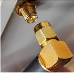
6. Hand tightened the antenna nut to the mount.
