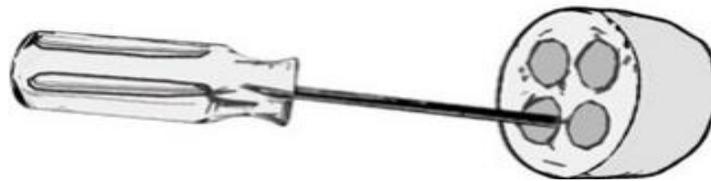
5. Pull 2 inches (5cm) of lead wire through the membrane for each one of the cables to be connected to the Multi-Channel Cable Node. Ensure that the number of membranes punctured matches the number of cables to be connected with a maximum of four cables per strain relief with one per membrane for a total of eight cables per Multi-Channel Cable Node.
