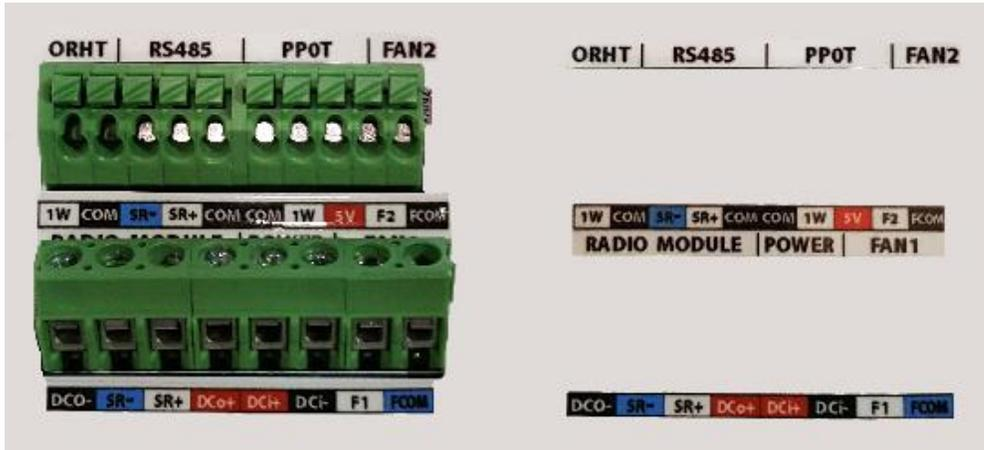
To correctly terminate all connections into the Fan Node, use the **Termination Connection Guideline Chart** below.
