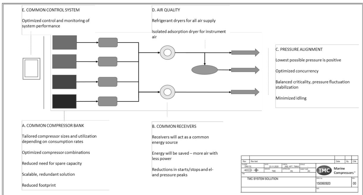
**Figure 2.** TMC System Solution® design principles.
