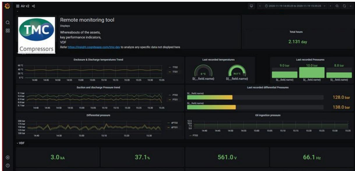
**Figure 3.** Proprietary TMC Smart Control data insight user interface for real time condition monitoring.
