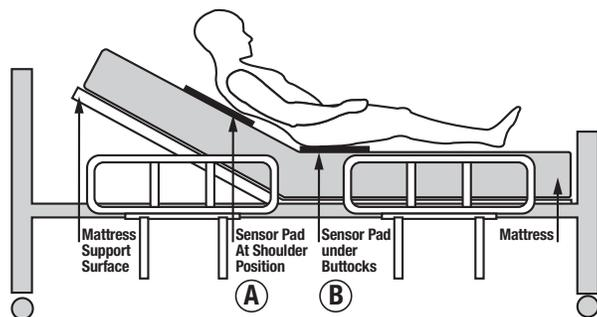
3. Place non-slip Posey Grip on mattress at area chosen for sensor pad. Place sensor pad over Posey Grip, across width of bed.
