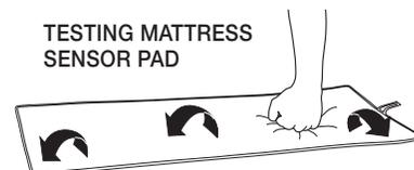
**WARNING** To reduce the risk of serious injury or death, **ALWAYS** follow these steps after putting the sensor pad in place and before leaving patient unattended (see instructions below). Do not use any alarm or sensor pad that does not alarm each time it is tested.
