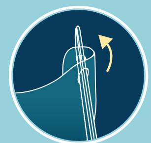
Slide lens forward into notches on frame
