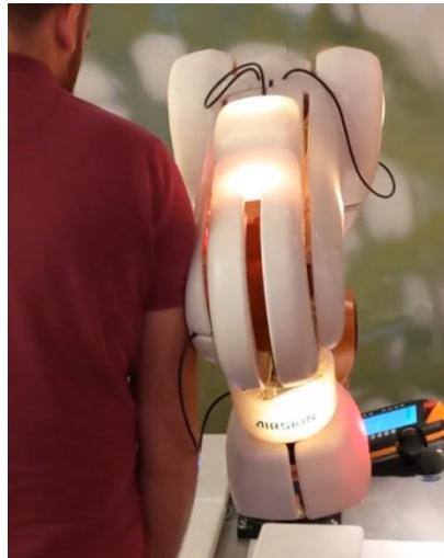
Barometric sensors monitor and detect air pressure change and trigger emergency stop. A piezo-micro-pump creates a small overpressure of ~400 Pa in the pads, to detect leaks.
