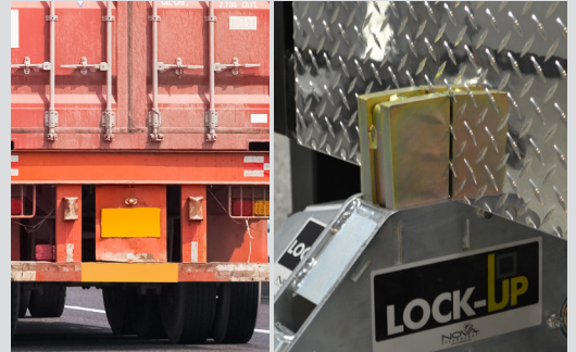
Vertical barrier ensures engagement by securing intermodal container chassis with rear impact guard obstructions
