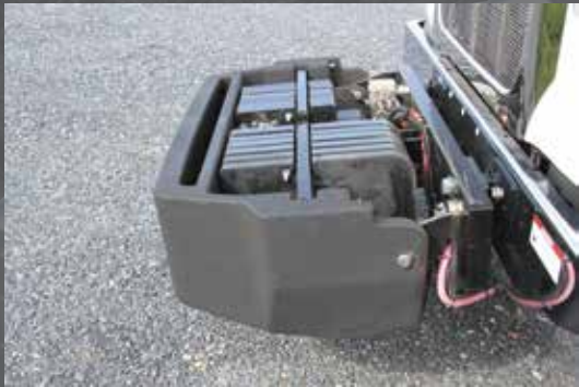
FRONT COUNTERWEIGHT 1001199186S 35T, 50T (Maximum 1980lbs of Counterweight Can Be Added) 1001213803 100LB COUNTERWEIGHT 1001213802 120LB COUNTERWEIGHT (Purchase One of Each to Balance the Weight)
