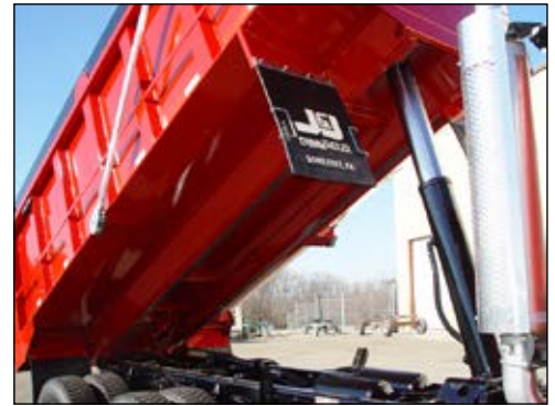
No crossmembers means lighter weight bodies.
