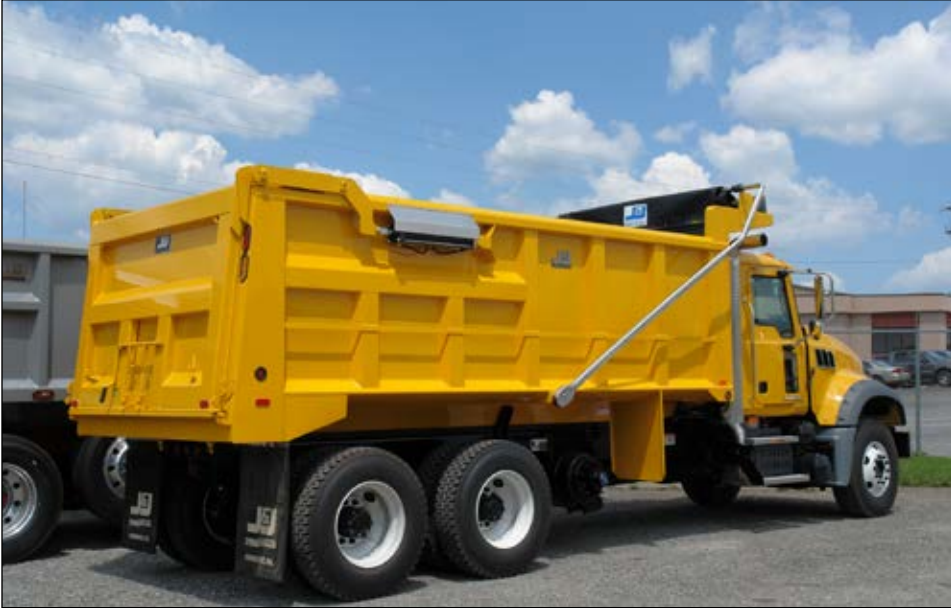
Sherwin-Williams Genesis® paint system provides a high gloss, extremely durable and resistant finish. All steel bodies are completely sandblasted for superior paint adhesion.
