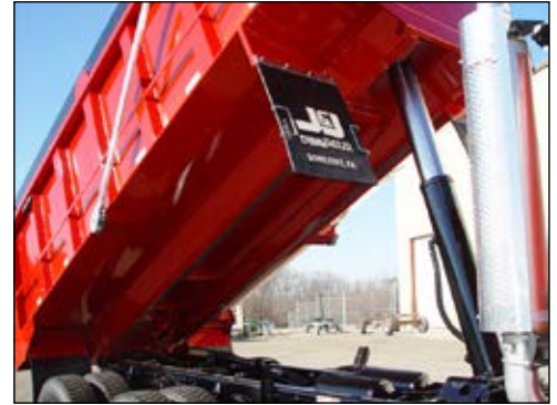
No crossmembers means lighter weight bodies.
