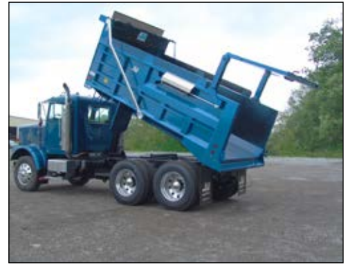
The air high lift tailgate option prevents tailgate damage from large objects and functions as a conventional tailgate for standard aggregate hauling.
