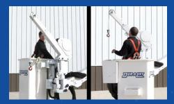
WORK FROM BOTH SIDES The new top mounted jib and winch allows the operator to rotate the jib to work on either side of the rotating basket.
