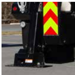
Telescoping rear stabilizers with integrated fold-down spade feet
