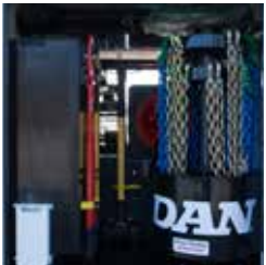
The innovative, patented Jerr-Dan chain carousel for effective, easy rigging access
