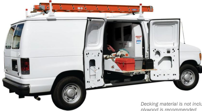
Decking material is not included, ¾" plywood is recommended
