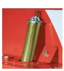
Return filters for the hydraulic oil come as standard, maintaining cleaner oil and reducing wear on hydraulic components. One of many details that help assure longer service intervals.
