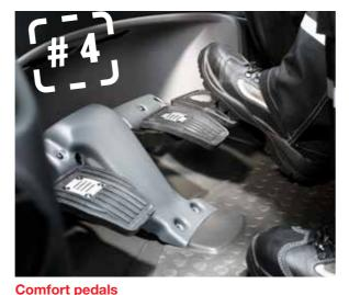
A new flexible and fail-safe pedal system with adjustable pedal angle to provide the best ergonomics and minimal strain on the foot. A floor-based solution with a hanging pedal feel.
