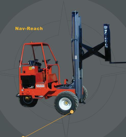
The optional "Nav-Reach" extension mechanism allows operators to unload a truck bed or trailer from one side
