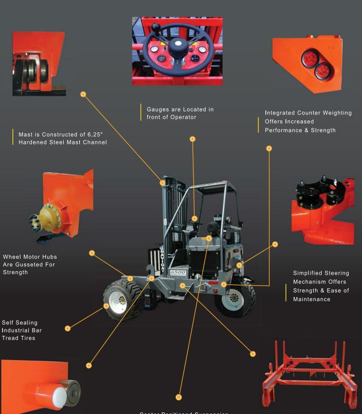
Adjustable Guide Blocks Keep Lift/Slide Carriages Straight in Frame Center Positioned Suspension Seat Provides Outstanding Comfort, Safety and Vision
