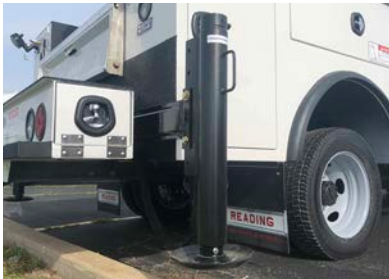
MANUAL/HYDRAULIC OUTRIGGERS Manual in/out (roller-bearing assisted), hydraulic up/down outriggers.
