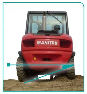
OSCILLATING REAR AXLE Ensures the tires stay on the ground traveling over rough terrain surfaces.
