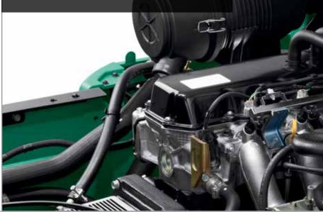
**Cool And Quiet:** The forklift's fan and radiator system is equipped with a horizontal cross flow cooling system to help keep the engine cool and functioning at peak performance. The corrugated design provides optimal heat exchange, while the aluminum core helps to prevent corrosion. The direct drive fan also reduces noise and necessary maintenance, benefiting your operators and your business.
