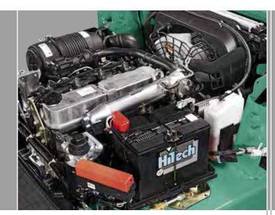
**Engine Protection:** Regulated by the Vehicle Control Module, the Engine Protection System keeps the truck running at desirable levels while helping to prevent damage to the forklift, saving you money. If any of the vital fluids become critically low, RPM levels are automatically lowered and the operator is immediately notified by a light on the dash display.
